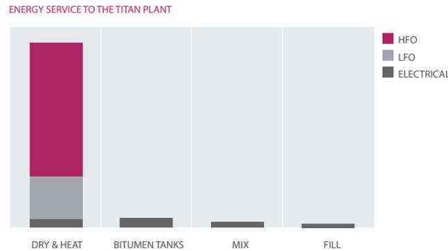
Figure 02. Stacked bar chart demonstrates the significant overall energy services to the four Tar plant processes
