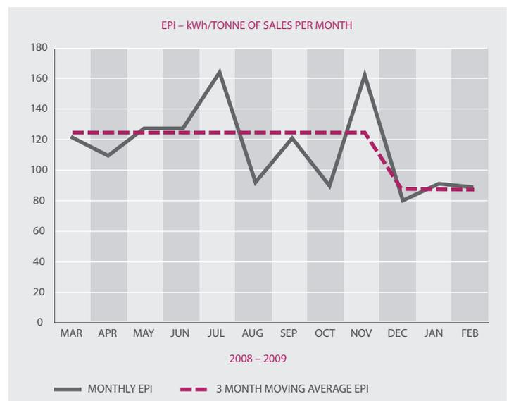
Figure 01. EPI showing energy consumed per tonne for the preceding 12 months and indicating a process shift between December and February. This reflects the savings derived from the reduction in rejected material.
